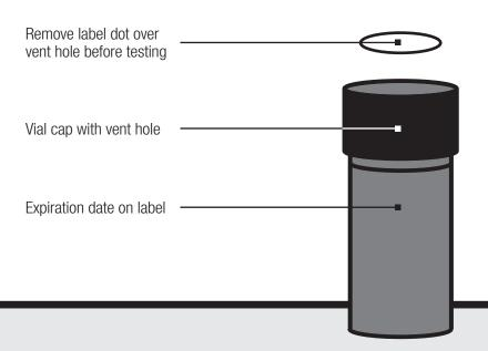
**NOTE:** Replace the Test Vial back in the nylon bag when not in use to extend the shelf life. Replace Test Vial when the green color is less than ½ full or at the time of the expiration date.
