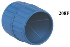
Reamer for 3/16" to 1-1/2" OD copper, aluminium and brass tubing. Hardened steel cutter blades. Reams both inside and outside edges of tube with 3 hollow ground cutters. Tough die cast body. Deburrs both clockwise and counter-clockwise. Fluted body is shaped to fit comfortably in palm.
